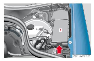
**1** Main fuse box in engine compartment
